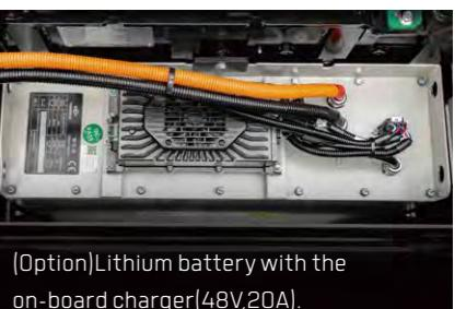
(Option)Lithium battery with the on-board charger(48V,20A).
